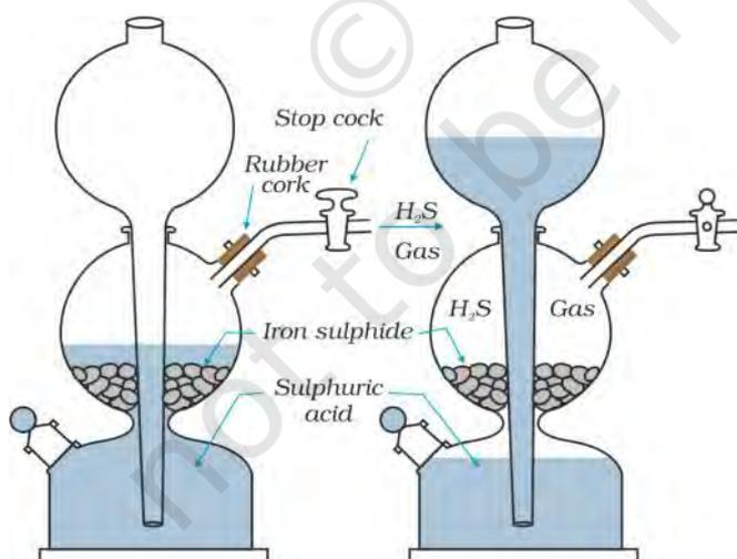
Fig. 7.8 : Kipp's apparatus for preparation of  $\text{H}_2\text{S}$  gas
