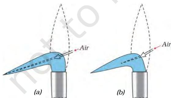
**Fig. 7.7 :** Obtaining oxidising and reducing flame
