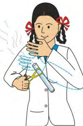
Fig. 7.9 : How to smell a gas
