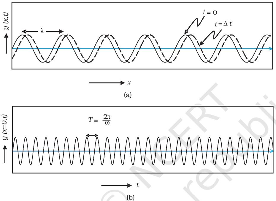
**FIGURE 10.17** (a) The curves represent the displacement of a string at  $t = 0$  and at  $t = \Delta t$ , respectively when a sinusoidal wave is propagating in the  $+x$ -direction. (b) The curve represents the time variation of the displacement at  $x = 0$  when a sinusoidal wave is propagating in the  $+x$ -direction. At  $x = \Delta x$ , the time variation of the displacement will be slightly displaced to the right.
