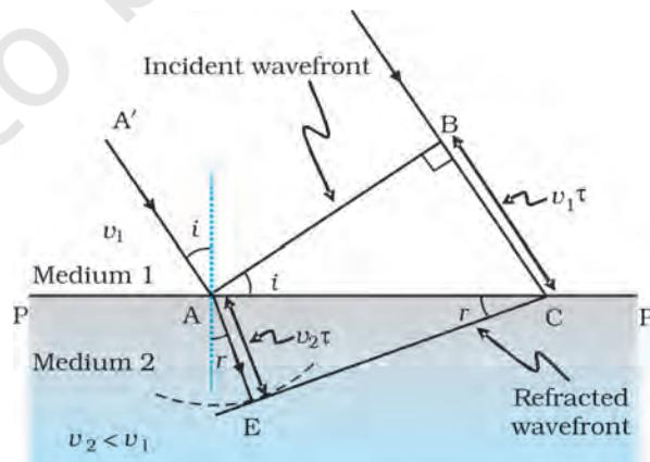
**FIGURE 10.4** A plane wave  $AB$  is incident at an angle  $i$  on the surface  $PP'$  separating medium 1 and medium 2. The plane wave undergoes refraction and  $CE$  represents the refracted wavefront. The figure corresponds to  $v_2 < v_1$  so that the refracted waves bends towards the normal.
