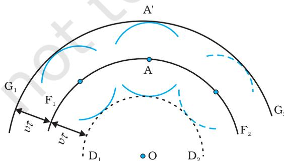
**FIGURE 10.2**  $F_1F_2$  represents the spherical wavefront (with O as centre) at  $t = 0$ . The envelope of the secondary wavelets emanating from  $F_1F_2$  produces the forward moving wavefront  $G_1G_2$ . The backwave  $D_1D_2$  does not exist.
