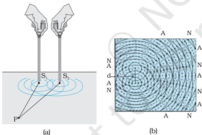
**FIGURE 10.8** (a) Two needles oscillating in phase in water represent two coherent sources. (b) The pattern of displacement of water molecules at an instant on the surface of water showing nodal N (no displacement) and antinodal A (maximum displacement) lines.
