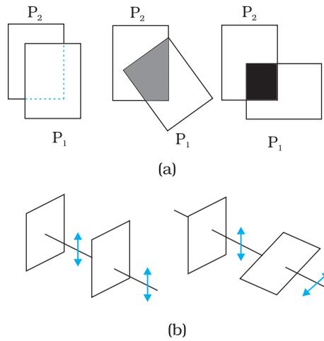
**FIGURE 10.18** (a) Passage of light through two polaroids  $P_2$  and  $P_1$ . The transmitted fraction falls from 1 to 0 as the angle between them varies from  $0^\circ$  to  $90^\circ$ . Notice that the light seen through a single polaroid  $P_1$  does not vary with angle. (b) Behaviour of the electric vector when light passes through two polaroids. The transmitted polarisation is the component parallel to the polaroid axis. The double arrows show the oscillations of the electric vector.
