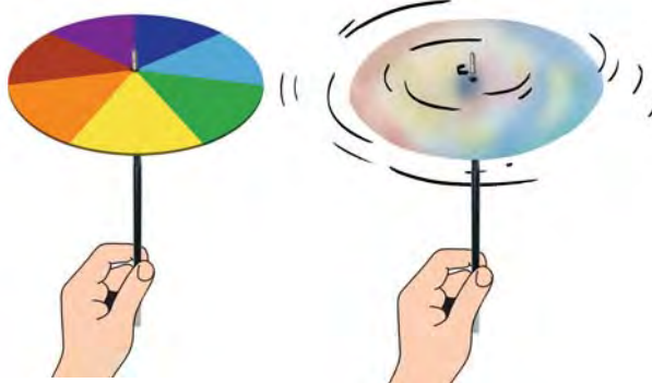
Fig. 7.12.4 (a) A disc with seven dours (b) It appears white by rotating
