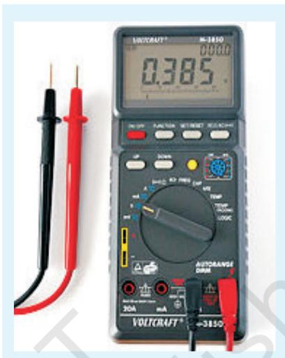
**Fig. A 4.1(b)** Digital multimeter
