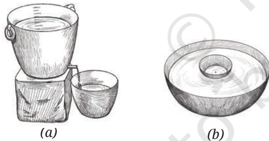
Fig. 8.2: A water clock (a) Water flowing out-type (b) Floating bowl-type
