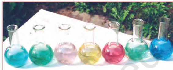
Fig. 4.5: Colours of some of the first row transition metal ions in aqueous solutions. From left to right: V^{4+} , V^{3+} , Mn^{2+} , Fe^{3+} , Co^{2+} , Ni^{2+} and Cu^{2+} .
